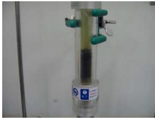
Figure 69. A column filled with algae/DME mixture (From Central Research Institute of the Electric Power Industry 2010).
