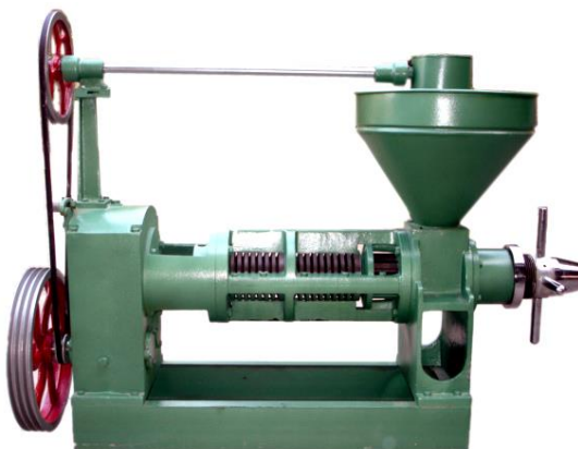
Figure 68. Commercially available expeller press using a screw device; motor not shown. (From Hunan Double Elephants Machinery Company 2013).
