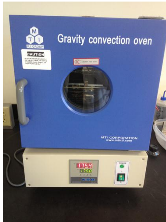
Figure 19. Gravity Convection Oven Used to Sensitize Samples
