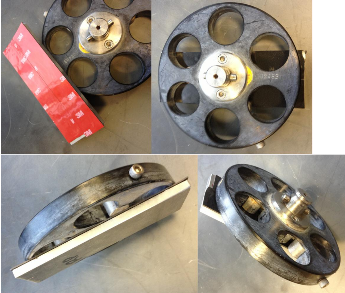
Figure 22. Image Showing Mounting Arrangement for Polishing Samples with the Automet
