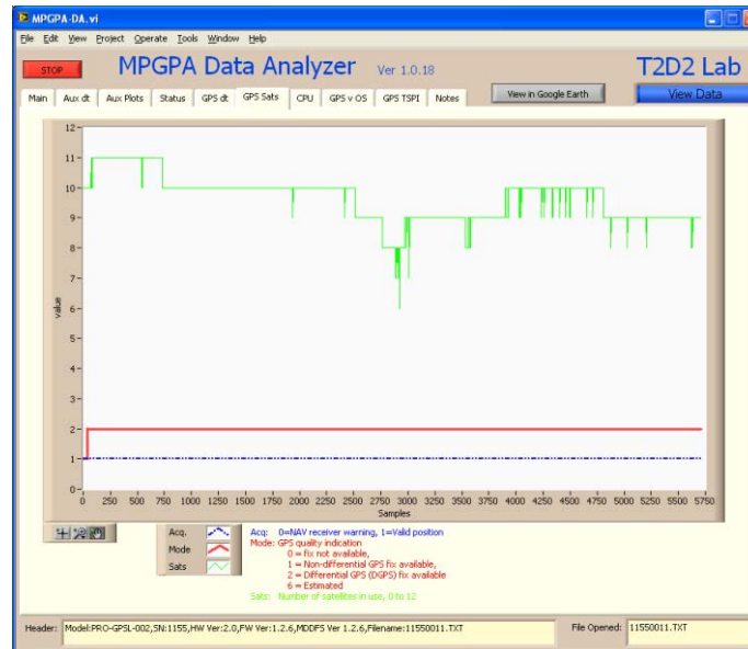
Figure 27. Notch Occurred While Moving GPS Over Survey Point, Not While Driving by Wind Turbine (No EMI Shield, Wind Turbine Starting and Stopping) (from Hynes, 2012, p. 24)
