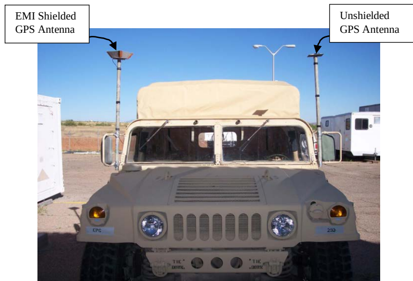
Figure 22. HMMWV Showing GPS Antennas Mounted on Each Side (after Hynes, 2012, p. 2)
