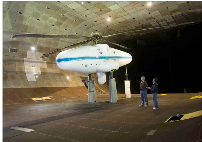
Figure 1. UH-60A Airloads rotor installed on LRTA in NFAC 40-by 80-Foot Wind Tunnel.
