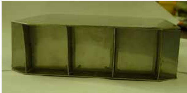
Geometry of the square honeycomb core: 5.5" X 5.5" X 1.6", Weight: 506g.
