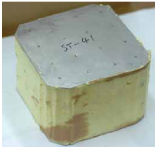
Geometry of NPR: 5.5" X 5.5" X 3.5", Weight: without foam: 398g, with foam: 540g
