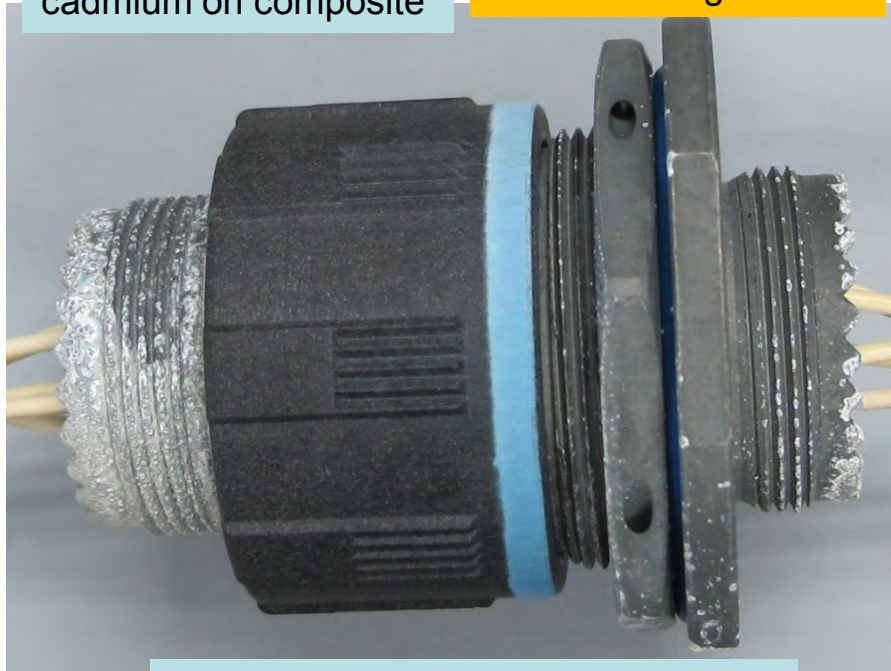
Cadmium corrosion product is evident especially on threads
