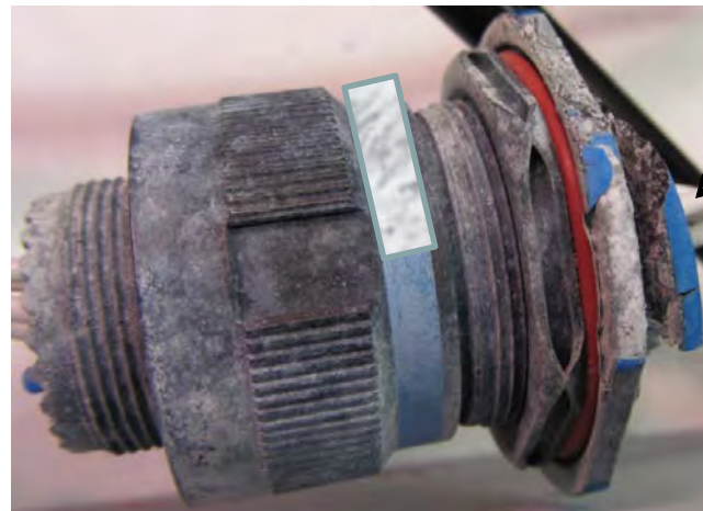
Plating flaking seen on several receptacle backsides
