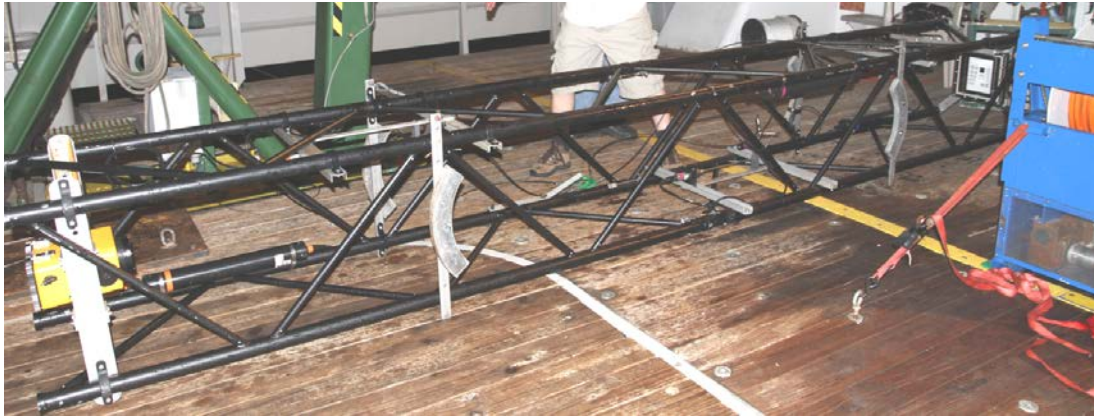
Figure 3. IMAST night deployment configuration: imaging camera and housing (left end of the frame); active target made out of iPad (right end of the frame). Notice the Vector and CT locations. Details on other sensors including Vector refer to text.
