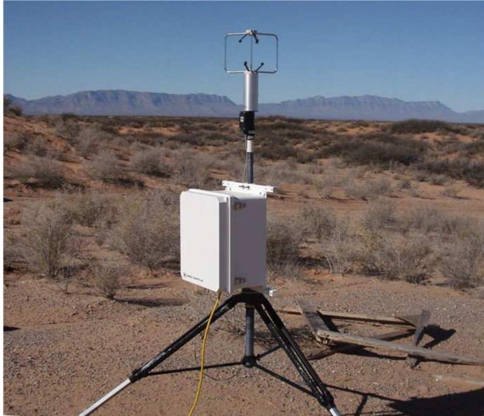
Figure 7. Downrange tripod with mounted 81000 RM Young sonic anemometer.
