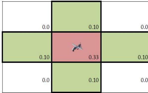
Figure 7. Sensor Model (Values represent sensor’s discretized effectiveness acquiring the potential information of cell)
