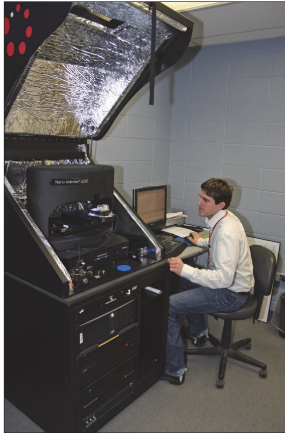
Figure 2. Agilent G200 nanoindenter used for nanomechanical testing.
