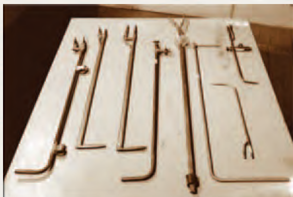
Multiple variations of Pitot tubes used at the Waterways Experiment Station.
