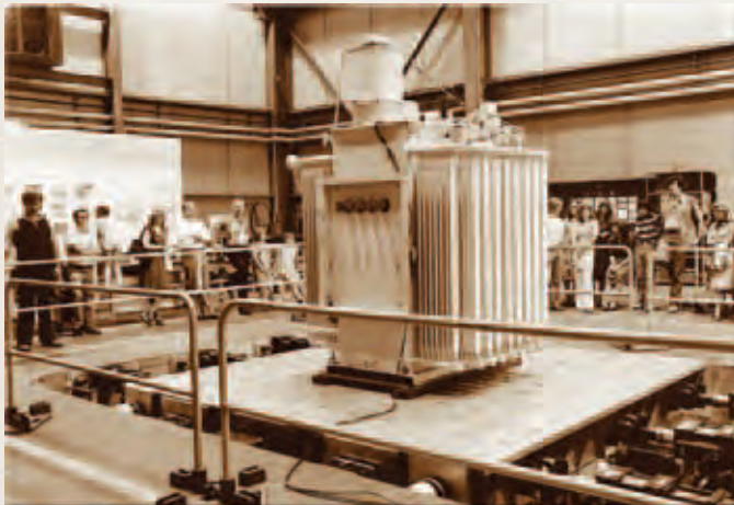
Biaxial shock test machine ready to shake a transformer.
