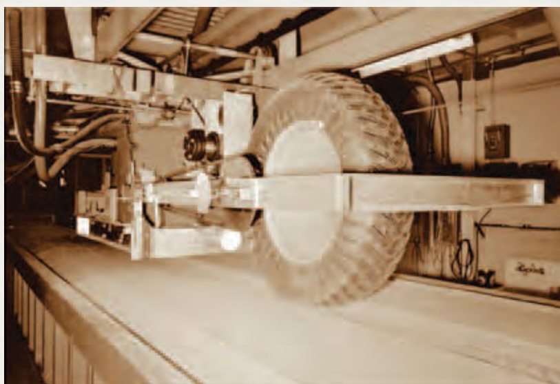
Lunar roving vehicle wheel undergoing test.
