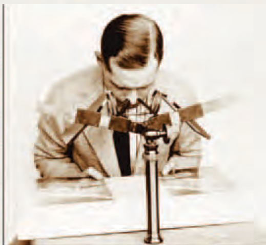
Using a stereoscope to bring images on adjacent photographs into coincidence. National Oceanic and Atmospheric Administration Photo Library.
