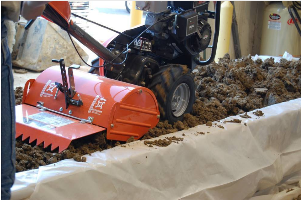
Figure 8. Tiller used to loosen the soil during soil preparation.
