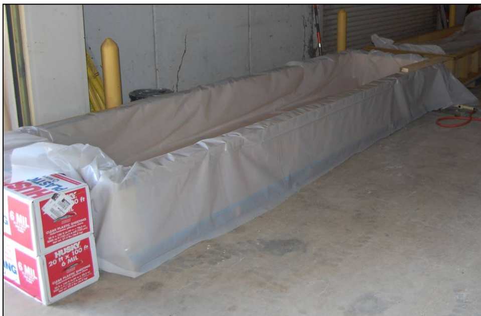
Figure 4. Wooden box with plastic cover for moisture protection.
