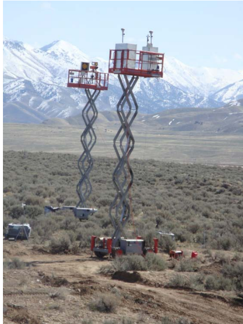
Figure 2-8. Two TEOMs and anemometer located on an elevated scissor lift (lift located closest to camera) at Tooele Army Depot, UT.
