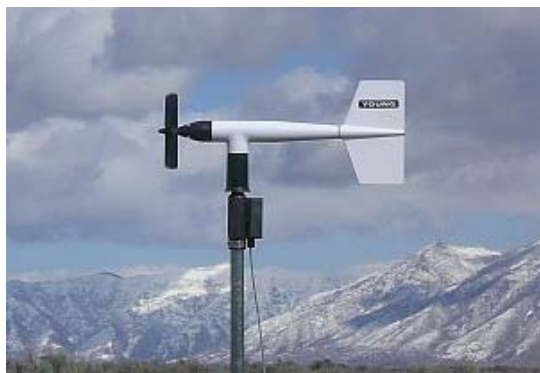
Figure 2-9. One of the two anemometers used during the Tooele Army Depot field campaign.
