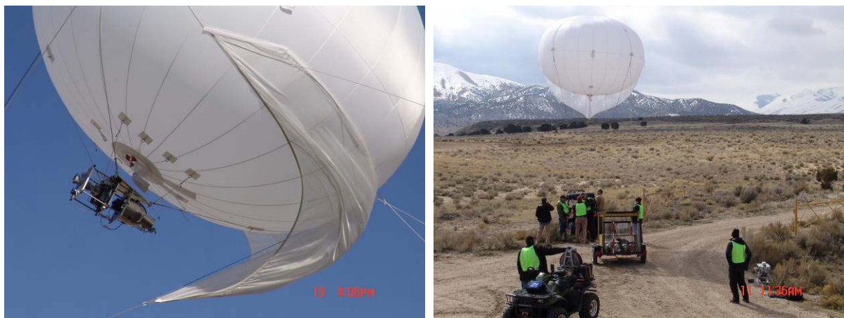
Figure 2-3. Balloon and Flyer (left) and balloon and ATV winch system (right).
