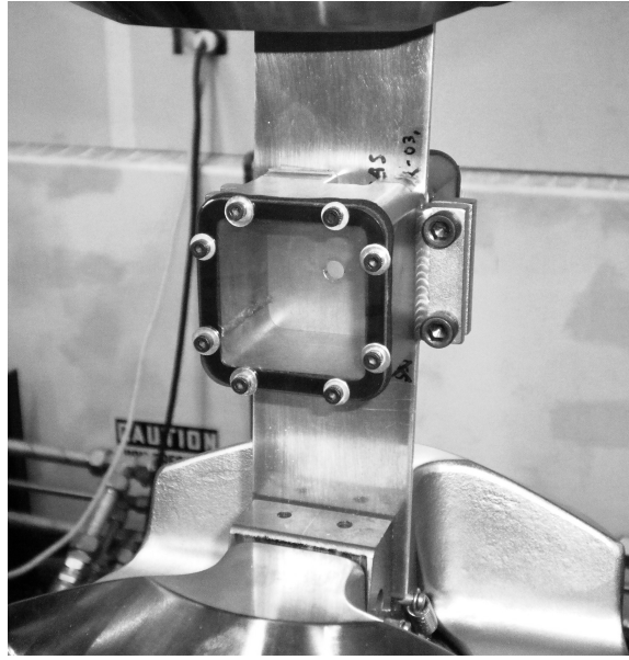
Figure 3.6: The water tight chamber used to expose the specimens to a saltwater environment while still allowing the crack growth to be monitored. The hole in the top of the chamber is used to fill them with saltwater.
