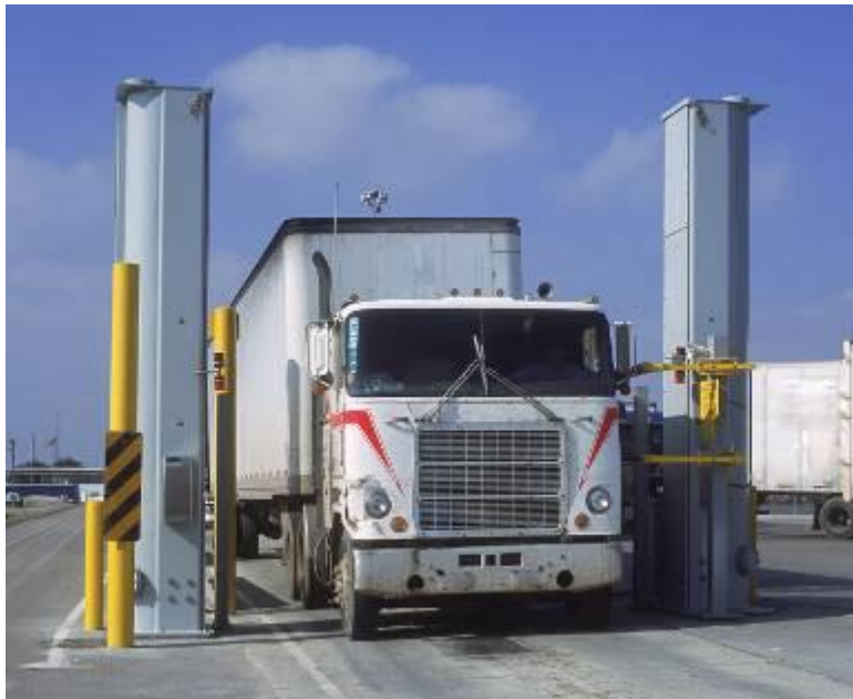
Fig. 1.6. A gamma-ray scanner system for use with transportation vehicles (SAIC, 2009).
