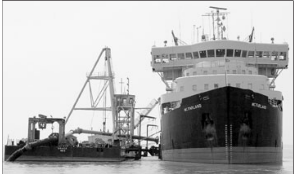
The McFarland hooks up to Mooring Barge #2 for direct pumpout to the disposal site
