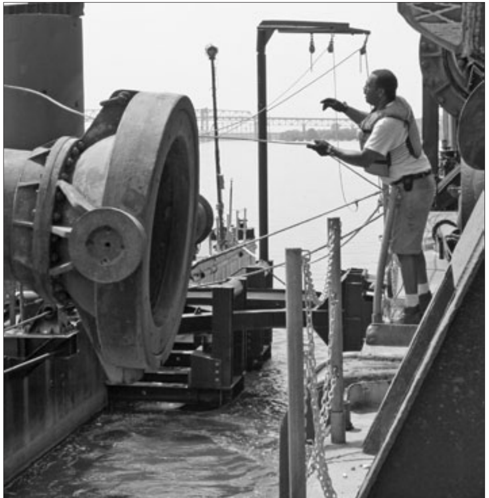
The McFarland hooks up to Mooring Barge #2 for direct pumpout to the disposal site
