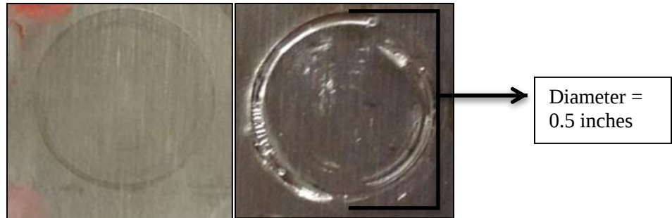
Figure 21: Galling coupons post testing at different loads. The sample on the left shows no trace of galling whereas the sample on the right galled.
