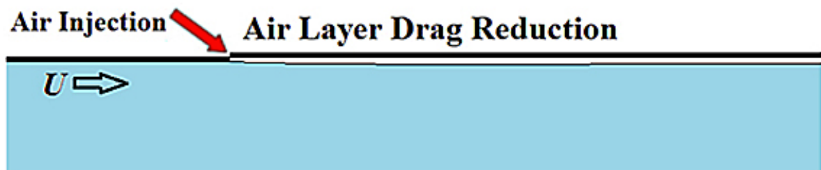
Figure 4: Air Layer Drag Reduction (Perlin and Ceccio 2013)
