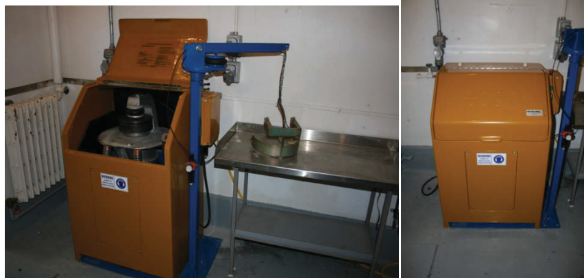
Figure 35. LabTech Essa LM-2 Ring mill, opened and closed.
