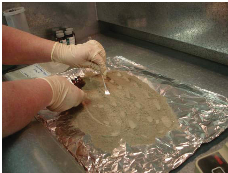
Figure 38. Build-up of a 10-g sub-sample using a systematic approach (30-increment).
