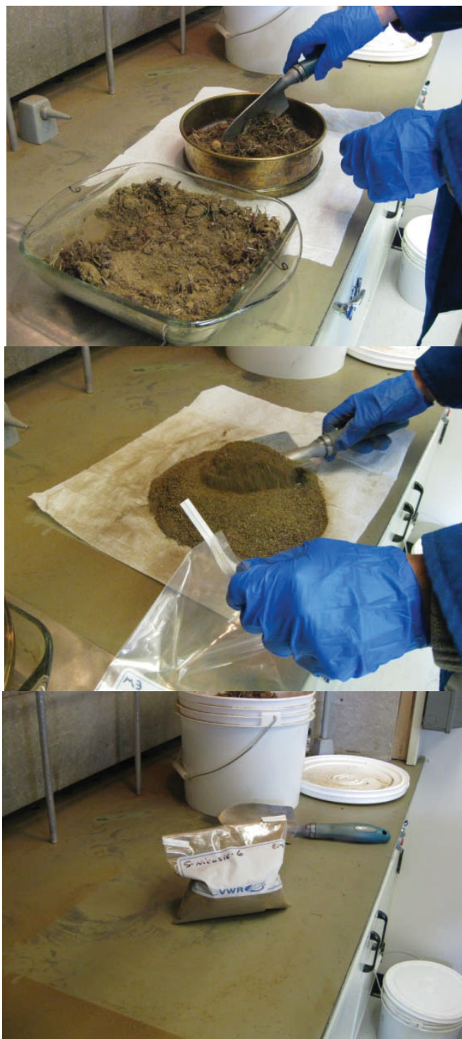
Figure 30. Sieving and storing the dried sample.
