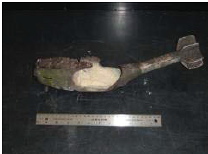
Figure 17. Resulting cracked UXO.
