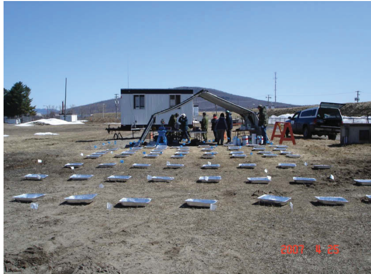
Figure 3. Propellant deposition trial – 7.62 mm.
