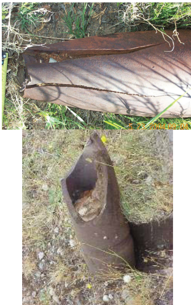
Figure 18. Cracked rounds found in an RTA.
