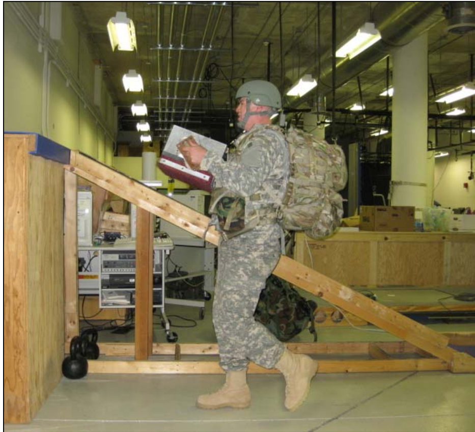
Figure 9. Soldier carrying a weighted box toward the platform while executing the repetitive box lift and carry test.
