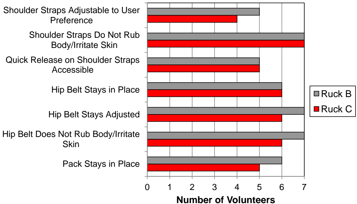
Figure 32. Number of volunteers agreeing with each statement pertaining to design features or functioning of the rucksacks ( N = 7 ).
