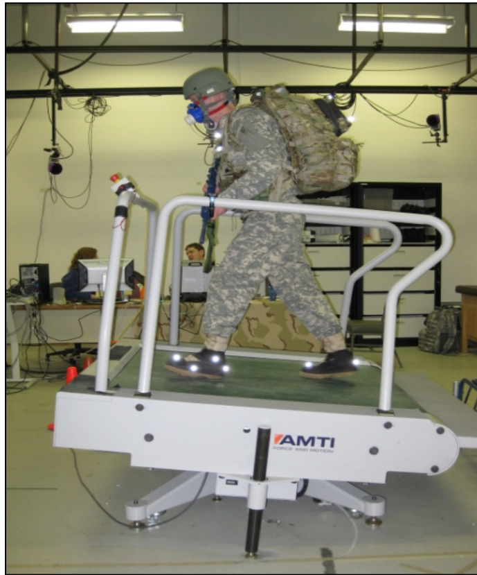
Figure 6. Soldier walking up a 9% grade on the force plate treadmill while oxygen consumption, kinematics, and kinetics were being captured.
