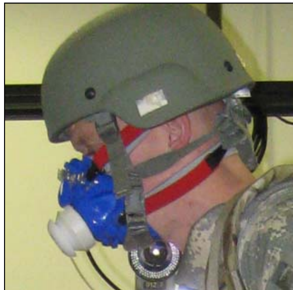
Figure 5. Soldier wearing the K4b 2 portable metabolic analysis apparatus used for measuring oxygen consumption.
