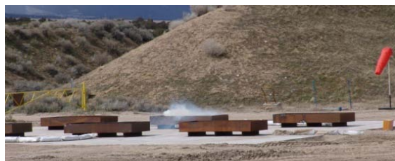
Figure 2-4. Concrete Burn Pad with six (left) and four (right) reusable burn pans.
