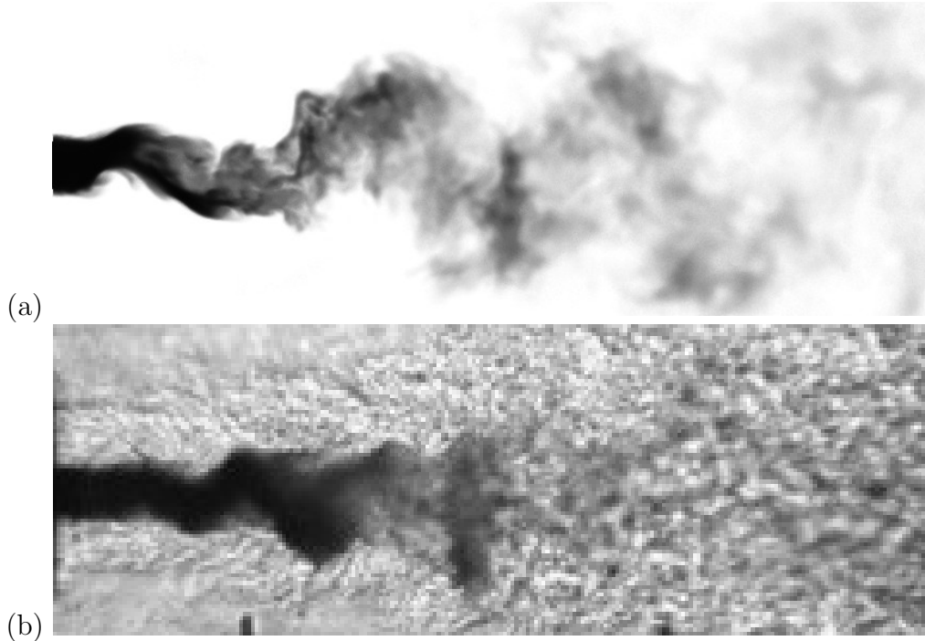
Figure 19: Case LarThin 1 Qualitative comparison between backlighting images from (b) experiment and simulation (a). Numerical results show density integrated over the line of sight.
