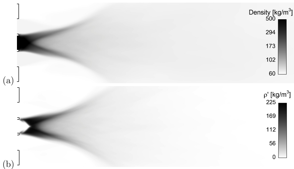
Figure 21: Case LarThin 2 . Longitudinal slice of (a) mean density and (b) rms density.
