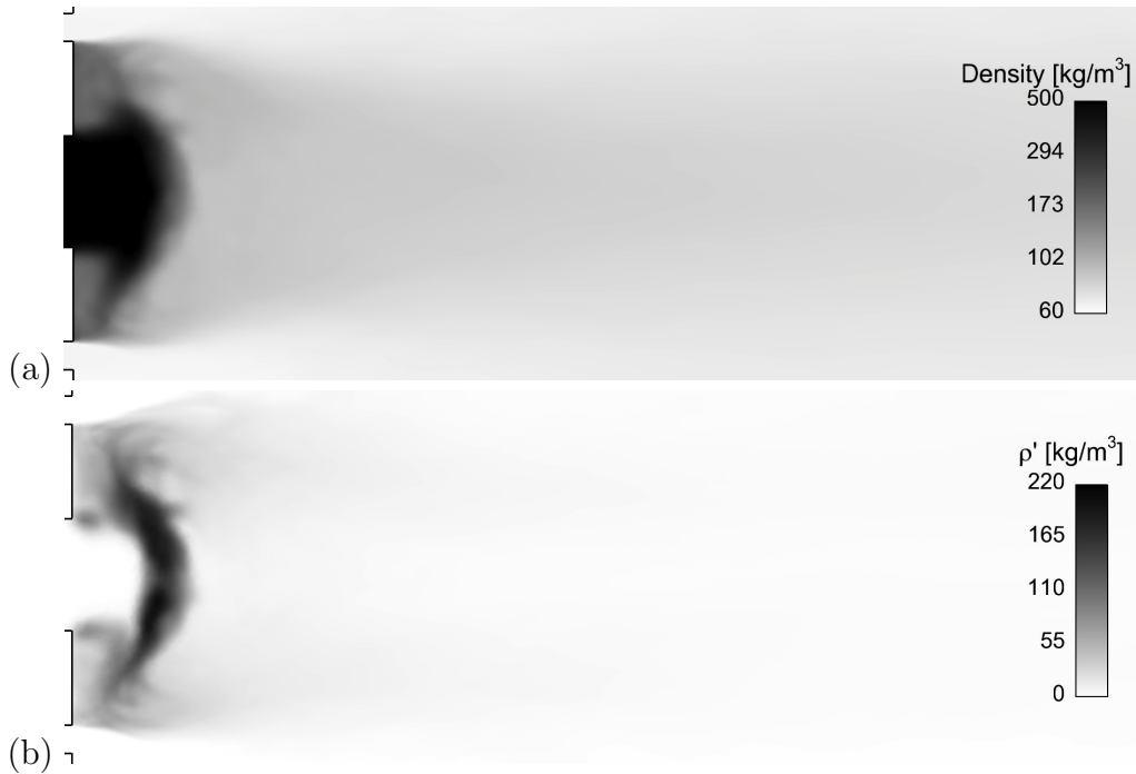
Figure 24: Case SarThick 2 . Longitudinal slice of (a) mean density and (b) rms density.
