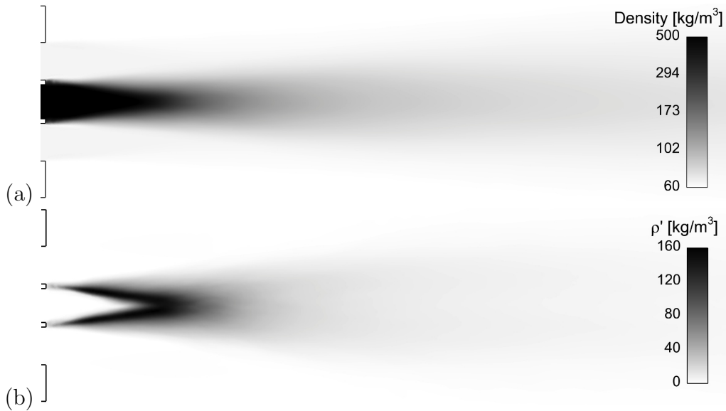
Figure 16: Case LarThin . Longitudinal slices of (a) mean density and (b) rms density.
