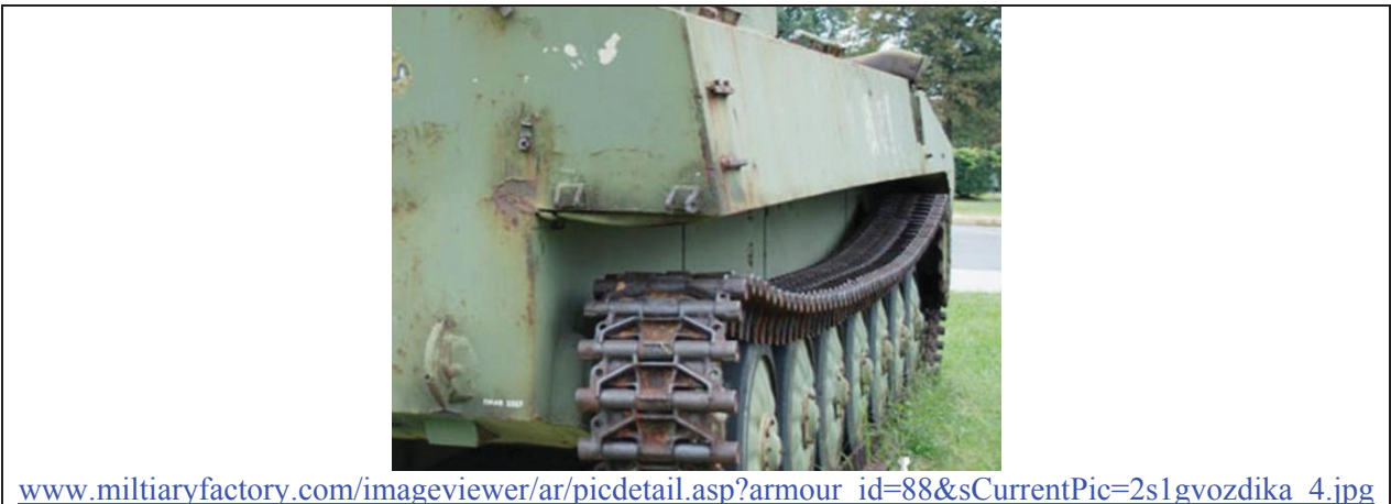
Figure 9: Gvozdika's track-and-wheel drive.
