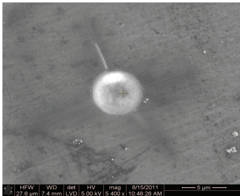
Figure 33. SEM micrographs of fused silica indented to 2000 nm.
