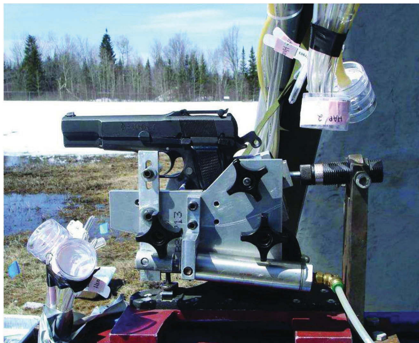
Figure 2. Browning pistol surrounded by air-monitoring cassettes and sorbent tubes.
