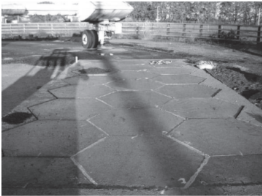
Figure 10. Accelerated pavement testing of hexagonal slabs in France (Kohler et al. 2007).
