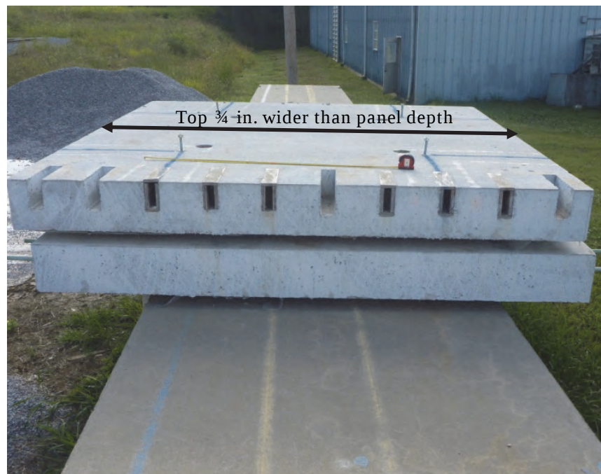
Figure 15. Dimensional problems with first precast panels.
