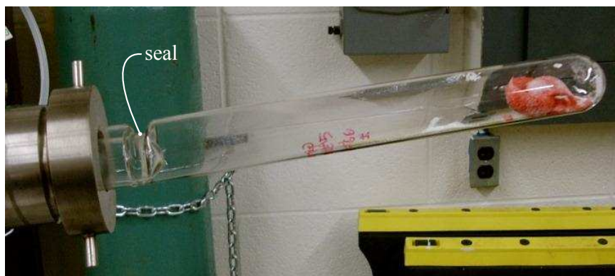
Figure 4.12. A sealed ampoule at the sealing port after the sealing procedure. This particular ampoule was an ampoule for the pre-growth polyethylene processing. The same ampoule-plug combination and sealing procedure were used for growth ampoules.
