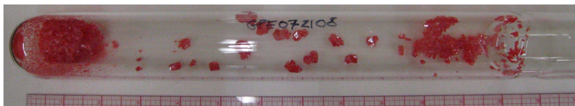
Figure 5.15. Growth with ultra high \bar{M}_w polyethylene, with T = 100^\circ\text{C} , \Delta T = 20^\circ\text{C} , and M = 2 \text{ wt-\%} .
