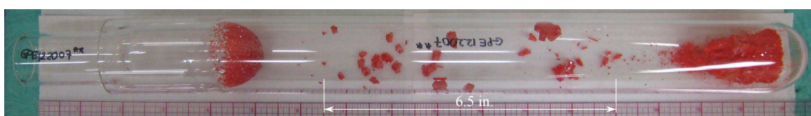
(b) T = 90^{\circ}\text{C} , \Delta T = 20^{\circ}\text{C} , M = 1 \text{ wt-}\%
