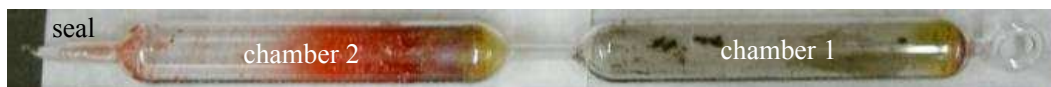
Figure 4.8. The double chamber ampoule (also seen in Fig. 4.5), after \text{HgI}_2 sublimation in static vacuum, from chamber 1 to chamber 2. Left behind in chamber 1 were black carbonaceous impurities.
