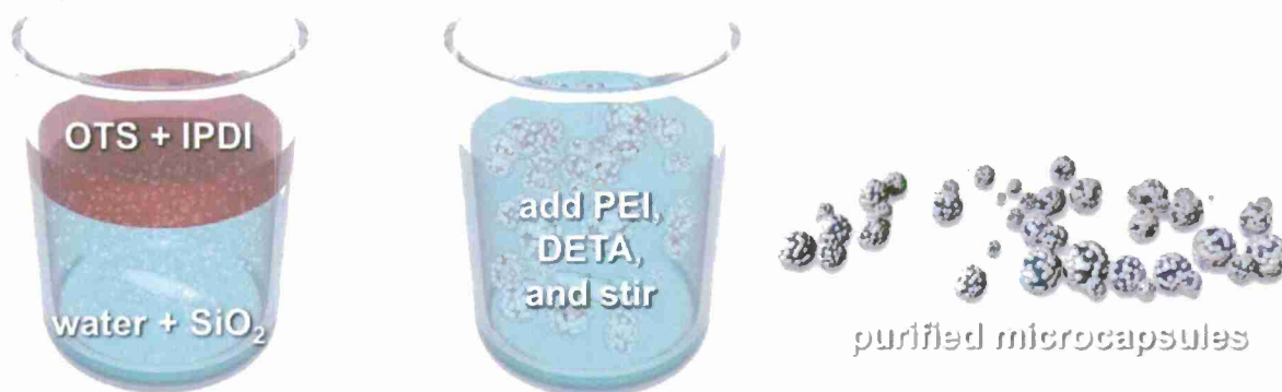
Figure 1: Schematic of microcapsule formation using a Pickering emulsion.
