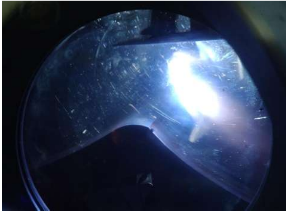
Fig. 20 Run#17 - Long exposure color photograph of laser-induced breakdown geometry at Mach 5.96; 2-D model at -7.5°; Shroud at -4° inclination.
