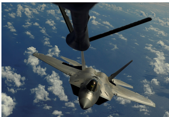
A U.S. Air Force F-22 Raptor fighter jet assigned to the 90th Fighter Squadron from Elmendorf Air Force Base, Alaska, approaches a KC-135 Stratotanker aircraft assigned to the 465th Air Refueling Squadron from Tinker Air Force Base, Okla., for aerial refueling.
