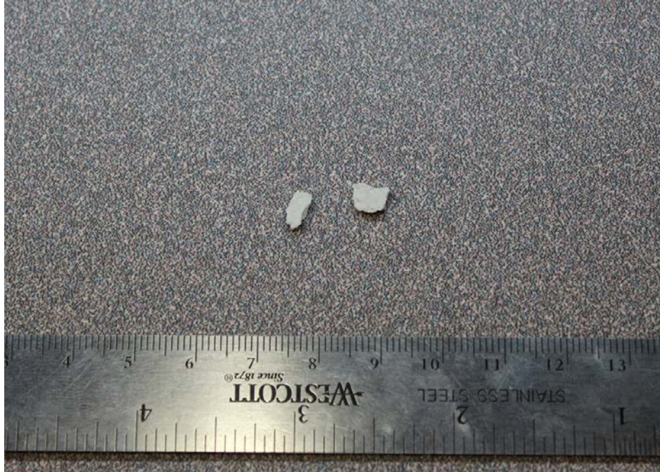
Figure 2.9. Coesite polycrystalline ceramic. Coesite is a high pressure phase of quartz.
