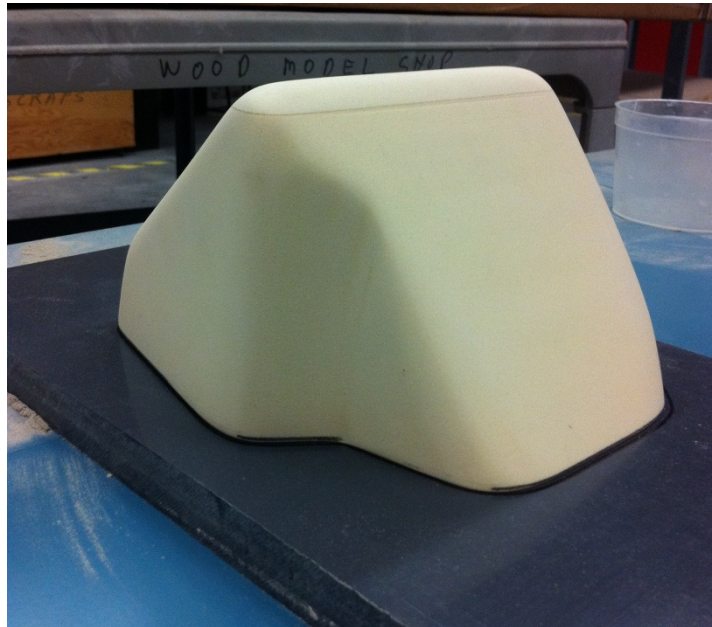
Figure 40: Crankcase Mold Mounted Prior to Priming
