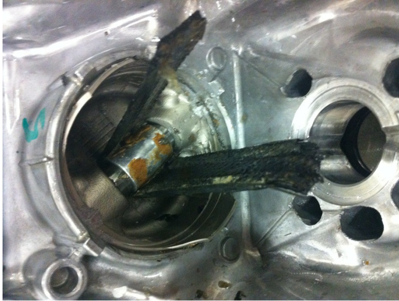
Figure 35: Catastrophic Failure of the CFRP Connecting Rod
