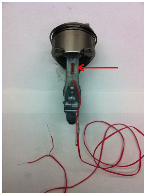
Figure 14: Mounted Strain Gage (Arrow) on the Stock Connecting Rod
