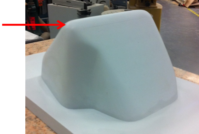
Figure 5: Shaped, Mounted, and Primed Mold for the Crankcase with Weak Spot Annotated
