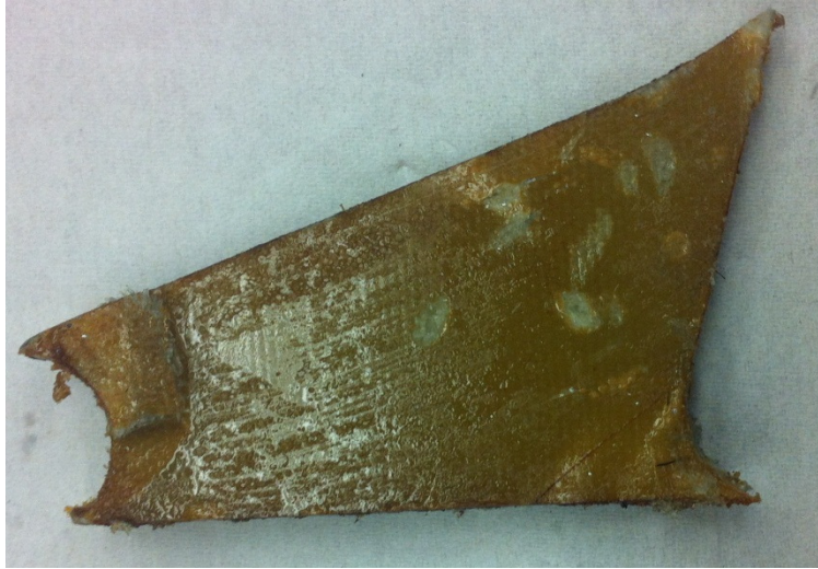
Figure 56: G10 Core after CFRP Connecting Rod Test
