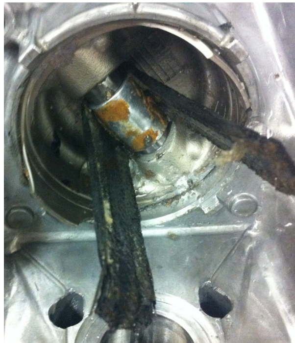
Figure 55: Failed CFRP Connecting Rod due to Bearing Sizing
