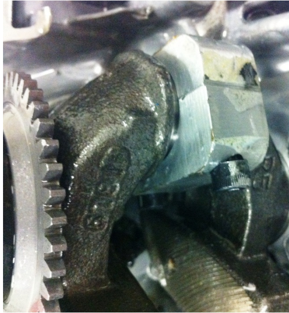
Figure 34: Seized Bearing Surface
