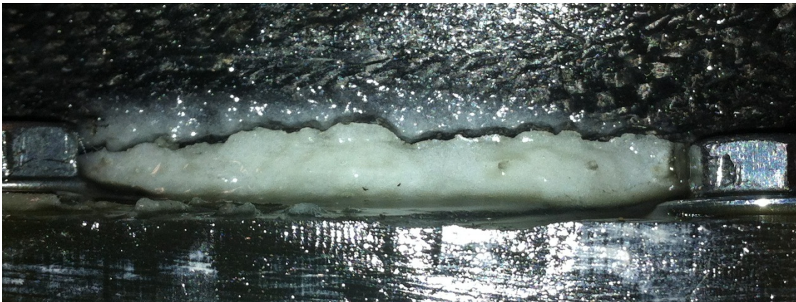
Figure 32: Cracked Epoxy Securing the Fiberglass Base to the CFRP Crankcase
