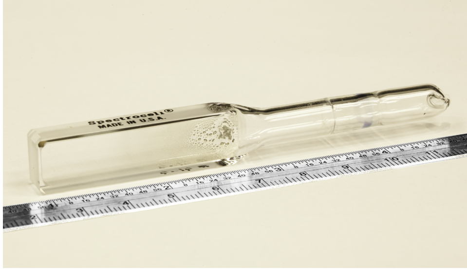
Figure 2. Spectra Physics DPAL Gain Cell. The cell has an overall length of 95 mm, of which 40 mm is the length of the reservoir. It has a height of 12.5 mm, a width of 7.6 mm and a wall thickness of approximately 1.5 mm
