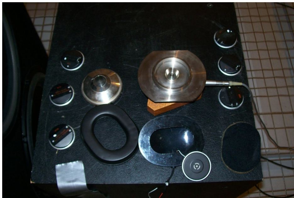
Figure 5. Earphone elements installed in a H-154/AIC earcup with ear cushion
