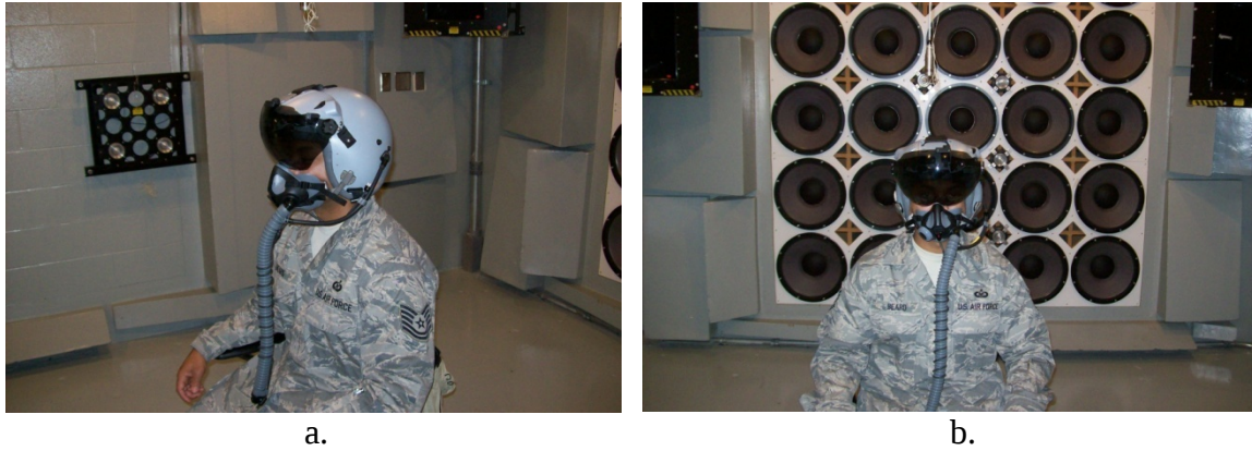
Figure 7. a. MIRE test subject b. MIRE test facility with speakers behind test subject
