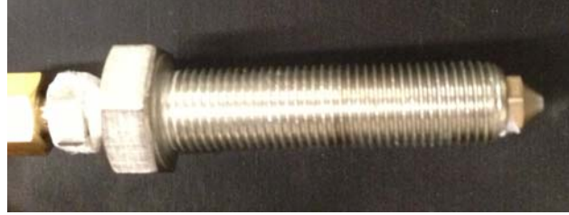
Figure 3.22: Fuel bolt assembly
