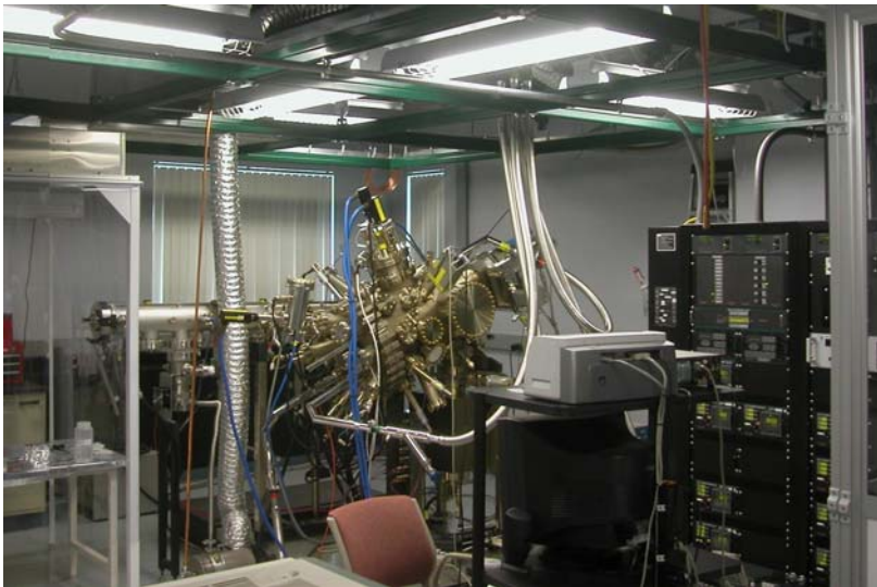
Figure 26: Veeco GEN-930 solid source molecular beam epitaxial growth machine
