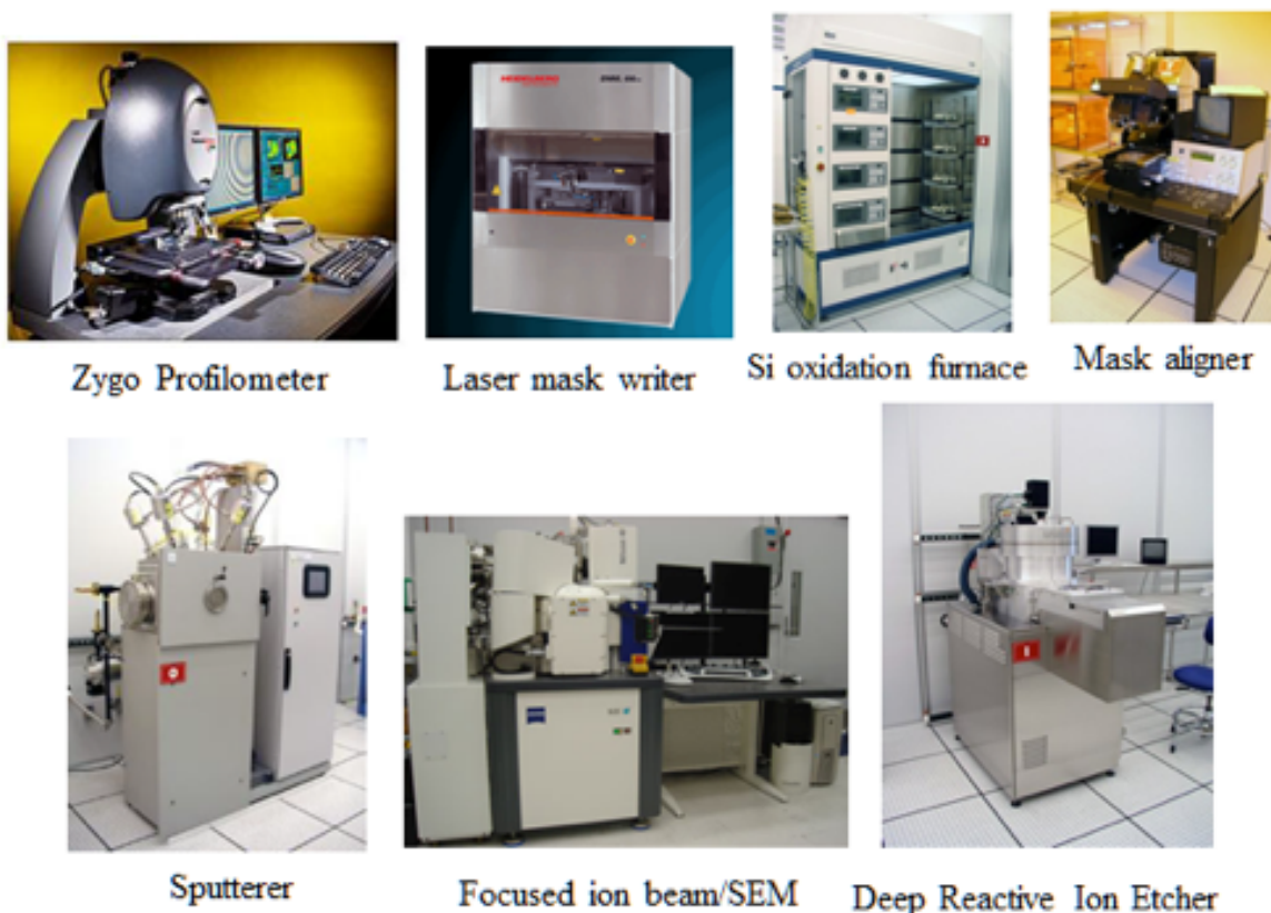
Figure 13: Nanofab equipment used at NIST CNST.
