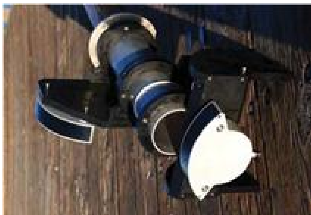
Figure B-8. Norbit FLS Dual Head set-up (left), associated surface instrumentation and control (right).
