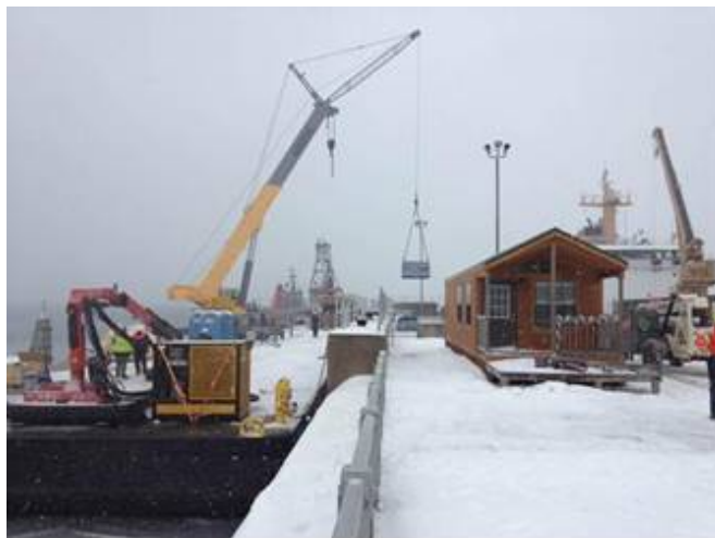
Figure 2. Crane on barge deck assisted in loadout of bucket skimmer and Aerostat IC container.
