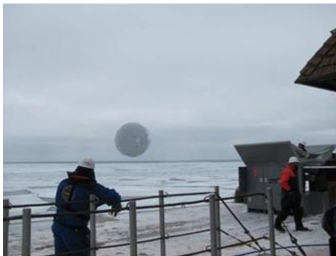
Figure 23. Aerostat IC balloon hindered by wind turbulence and eddies upon initial launch.
