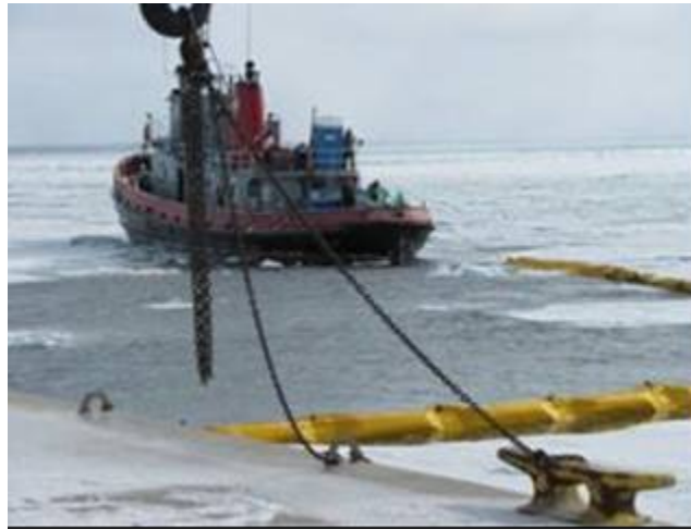
Figure 10. Tug towing American Fireboom MKII boom while being deployed from barge deck.
