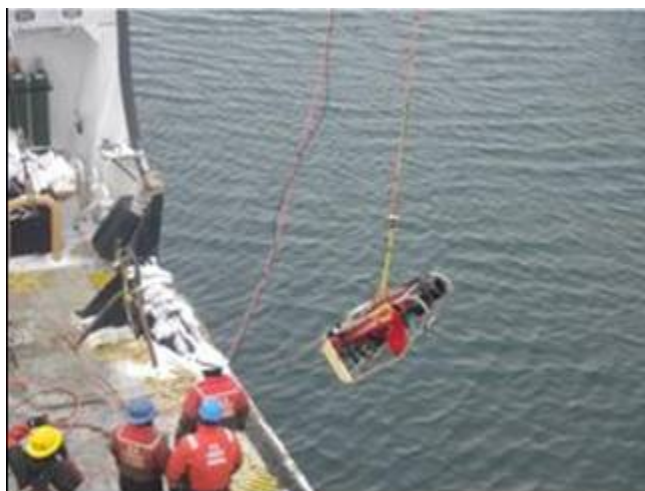
Figure 31. ROV being launched by crane from the deck of CGC Hollyhock.
