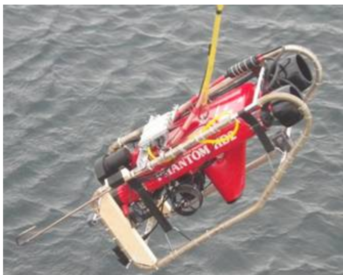
Figure 32. Close-up of ROV showing jury-rigged “shepherd’s crook” recovery hook (lower left of image).
