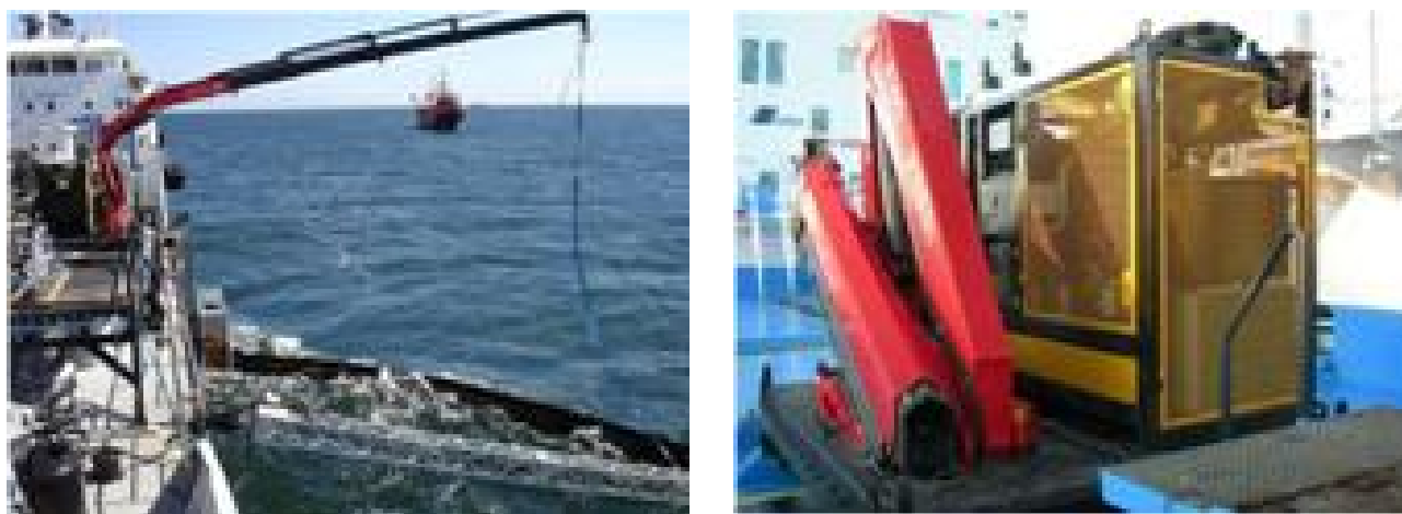
Figure B-9. Fassi crane in operation (left), Fassi crane and power pack on a 10' flat rack (right).
