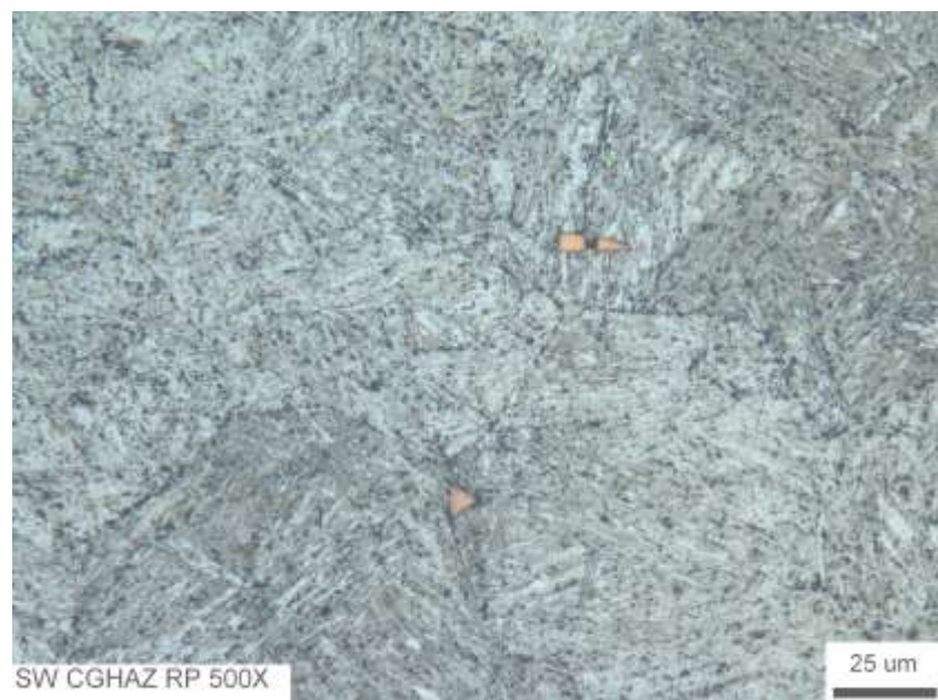
Figure 20 Single wire GMA coarse heat affected zone, root pass, original magnification 500x
