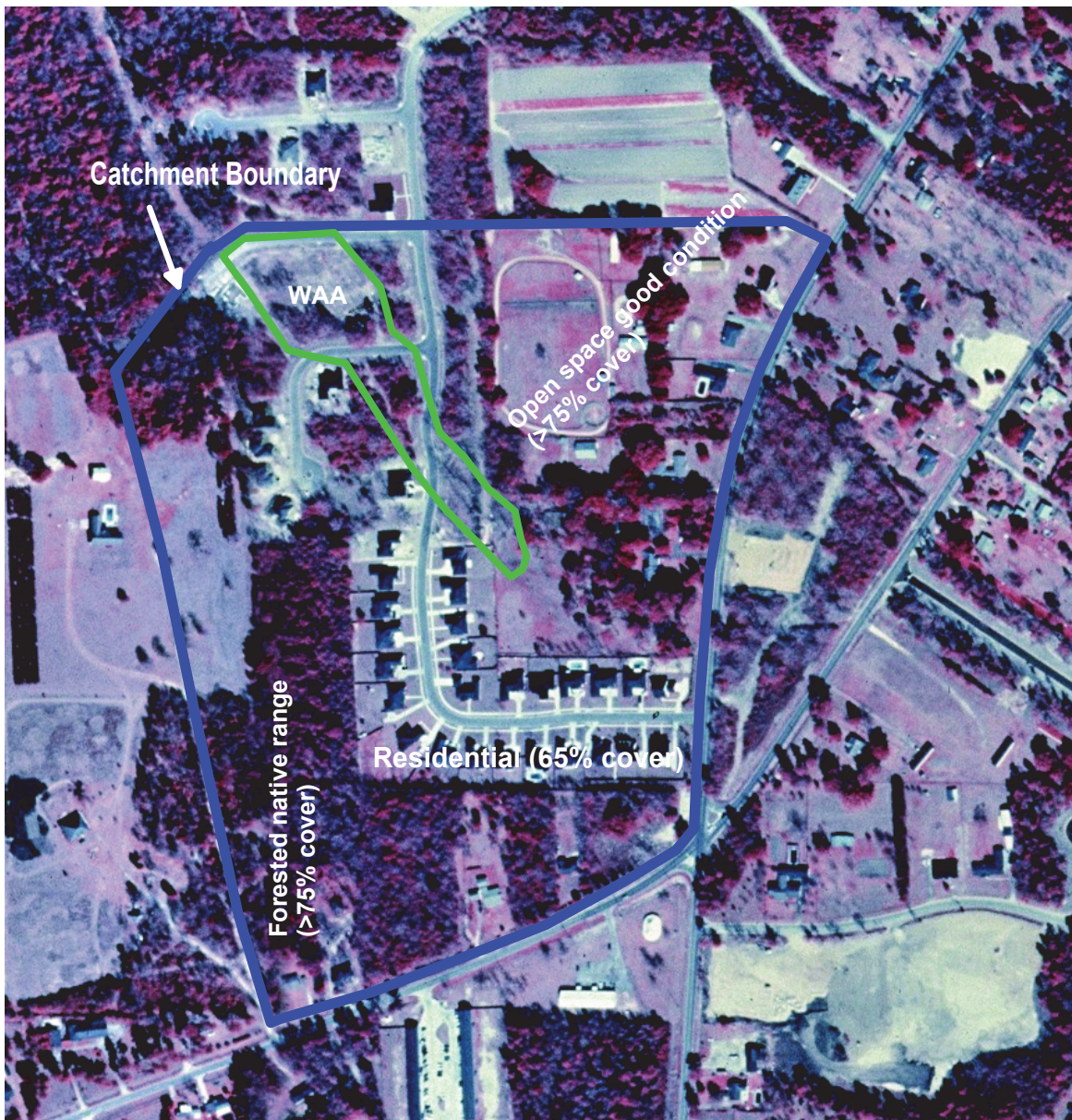
Figure D1. Aerial photograph illustrating the cover types found within the catchment of a wetland.
