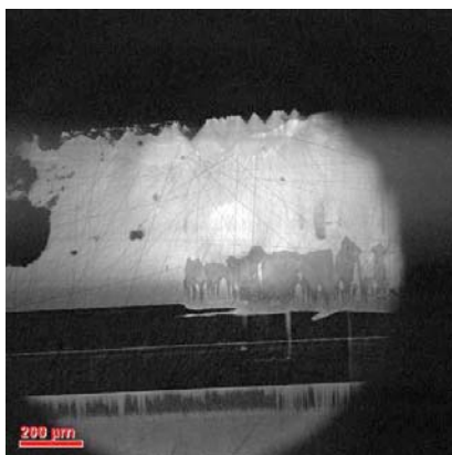
Fig.4. a) Panchromatic CL image of crystal B showing typical defects in c^- (top) and c^+ (bottom) crystal sectors.
