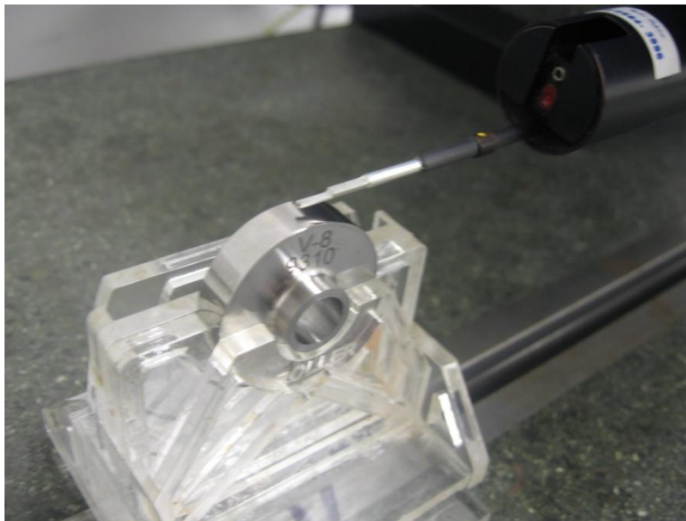
Figure 14. A disk (a) and roller specimen (b) being measured on the surface roughness profiler.
