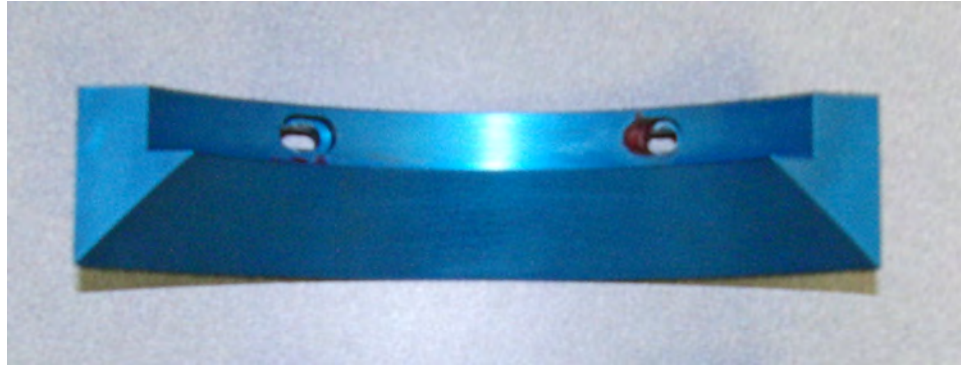
Figure 2.6: Wedge Cavitator used for Unswept Fin Testing
