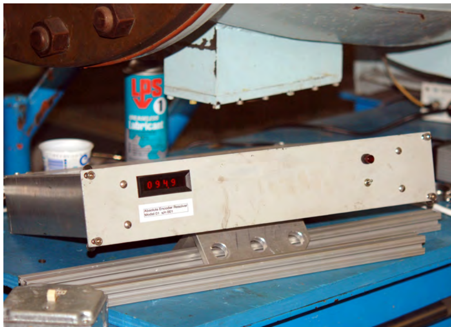
Figure C.9: Encoder resolver used to monitor fin's angle of attack.
