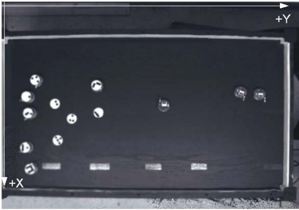
Figure 1: Overhead view of Khepera-II arena. Image taken from Cognex Insight 5400 machine vision sensor, showing several Khepera-II robots with unique identifier IDs (for truth measurements).
