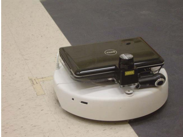
Figure 8. LATEST CONFIGURATION OF CREATE ROBOTIC AGENT, USING DELL MINI10 NETBOOK, LOGITECH QUICKCAM PRO 9000, AND HOKUYO URG-04LX-UG01 SCANNING LASER RANGEFINDER.
