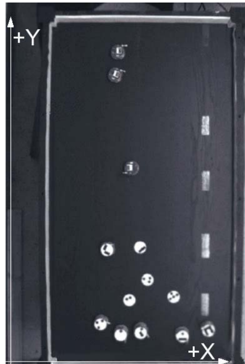
Fig. 2. Sample overhead image from Cognex 5400 camera of a rectangular arena with Khepera-II robots extending above a planar surface.
