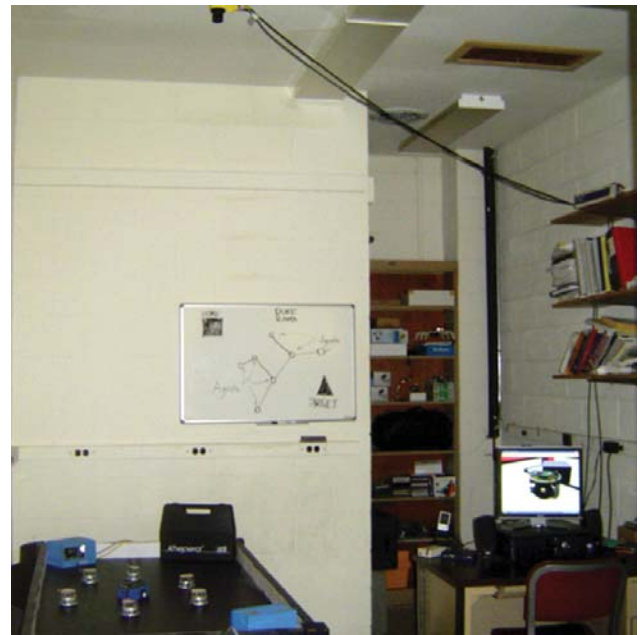
Figure 6: View of the Khepera-II lab space, showing relative locations of Cognex Insight 5400 camera and dual SICK LMS400 ladar sensors.
