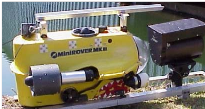
Figure 3-1. DIDSON attached to an underwater ROV.
