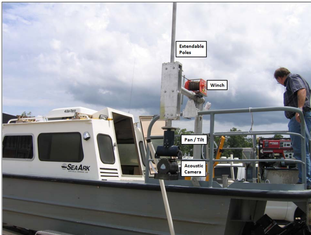
Figure 1-2. Acoustic camera mounted on a survey boat.
