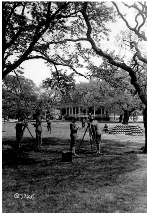
Figure 293: "Enlisted specialists school, Master Gunners' class" (Making a traverse by means of a transit.), 1918 (NARA RG 111 SC Box 69 9826).
