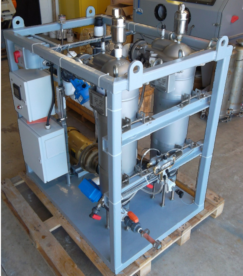
Photograph of the p3SFS showing filter housings, power box, controller, and main disconnect switch. Components are identified and details of the operation are provided in Drake et al., 2012.
