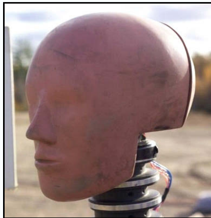
Hybrid III headform was developed by GM and used in automotive occupant safety
