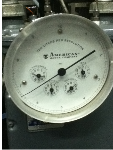
Figure C.5: Flow Meter Used to Calibrate Fuel Supply
