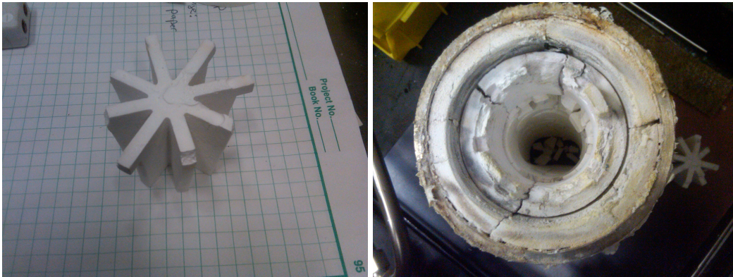
Figure 3.5: Flow Straightener and Transition Section
