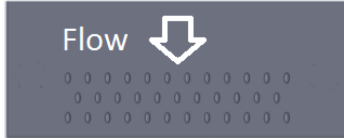
Figure 3.12: Triple Row of Cylindrical Holes Cooling Configuration
