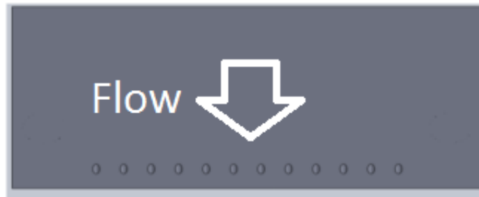
Figure 3.11: Single Row of Cylindrical Holes Cooling Configuration
