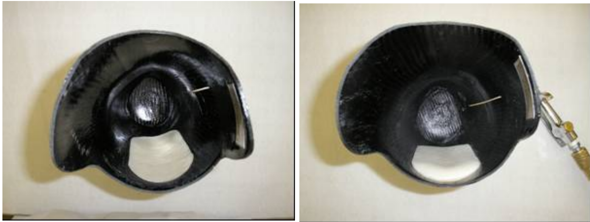
Figure 8: SMP foam pad fully compressed (left) and recovered (right).
