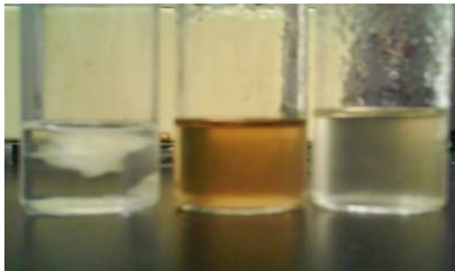
Fig 1: Photographs taken to observe thermally reversible cross linking behavior of modified epoxy with BMI. The cross-linked polymer was insoluble in DMF at room temperature (a), soluble at 130 °C and re-cross-linked at 45 °C.
