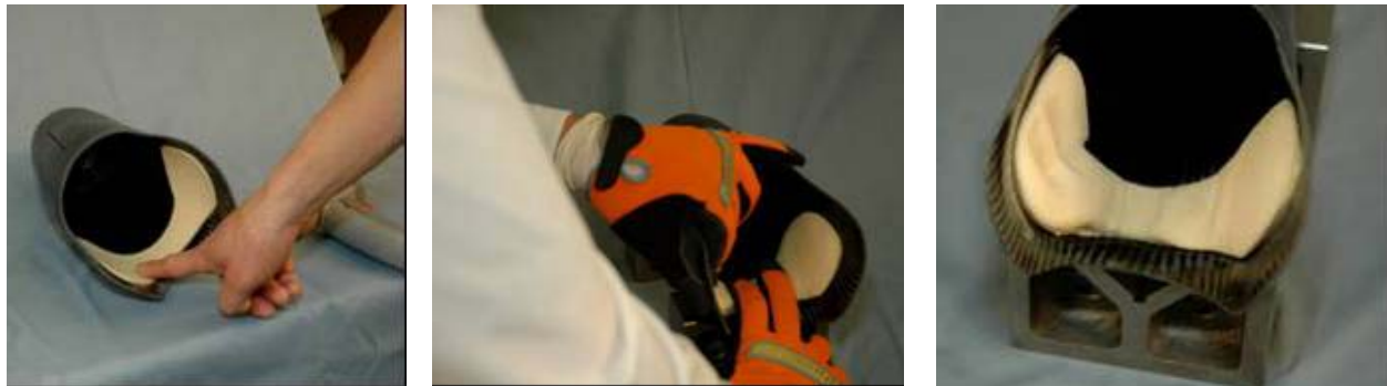
Figure 10: Left foam in the original none deformed state, center, foam heated and deformed locally, right, foam rigid in its locally deformed state.
