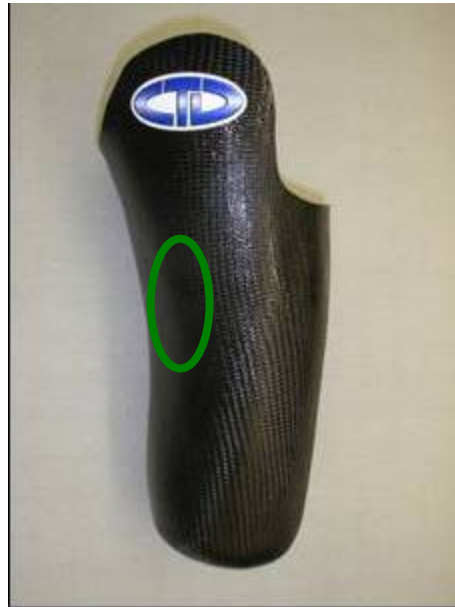
Figure 4: Area of socket thinning.
