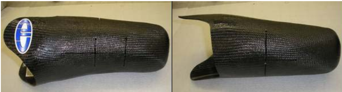
Figure 5: The anterior slotting of the socket (left), posterior slotting of the socket (right)
