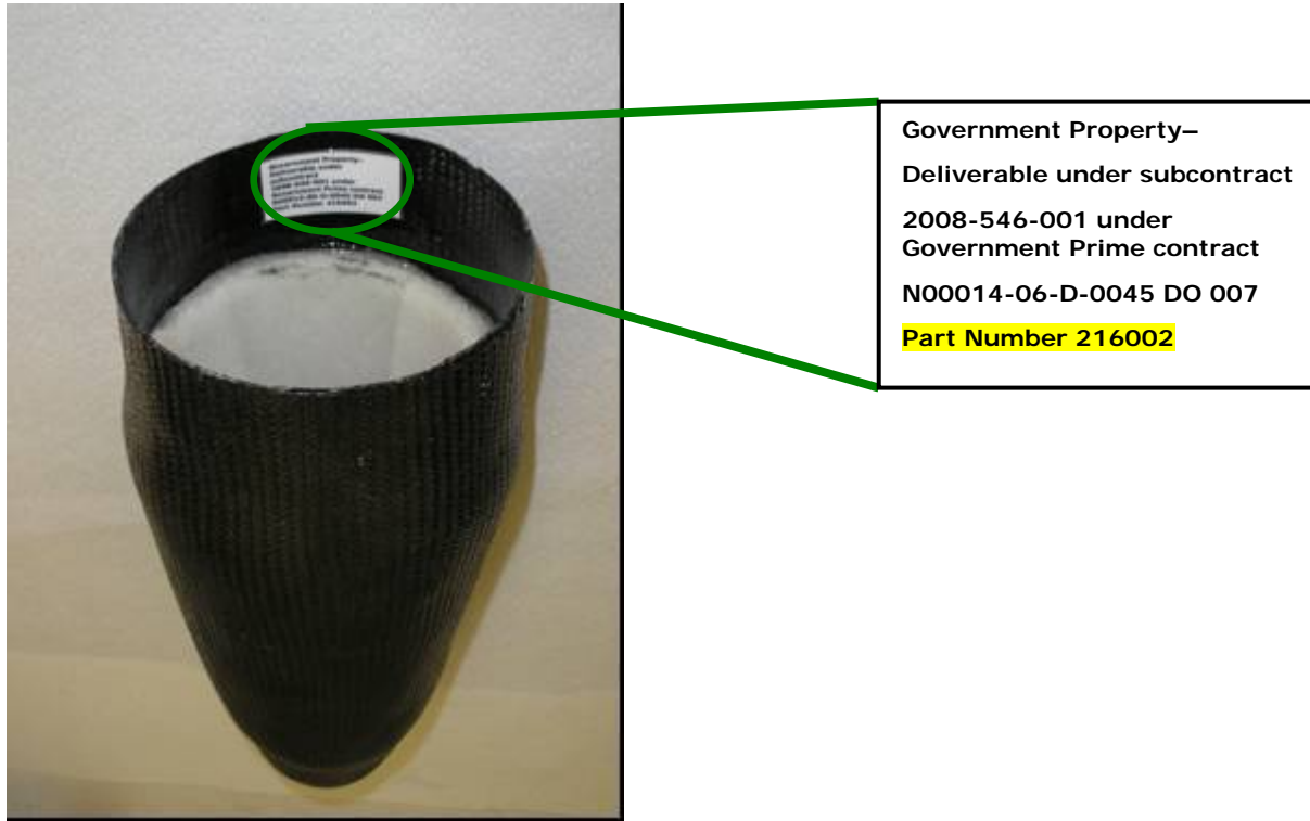
Figure 4: Example of part identification tag.
